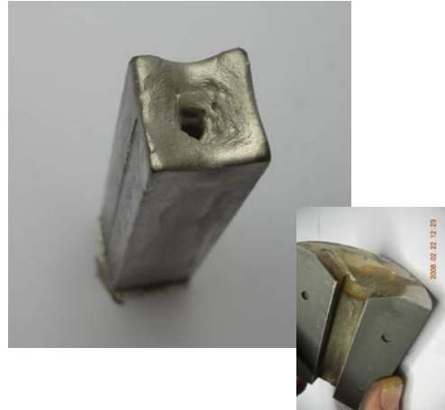
Observation of solidification shrinkage on top of an as-cast ingot
