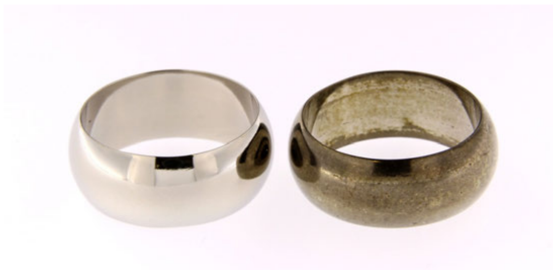
Figure 61 Ring (B) before and after industrial anodizing treatment.
