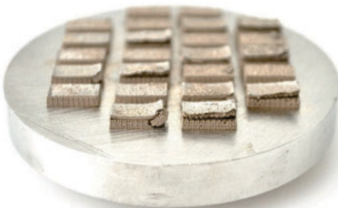
Figure 3 Example of samples with the ends rising and supports coming off.
