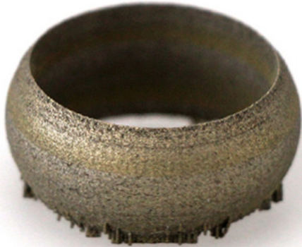
Figure 34 Solid ring printed with alloy (2) and power of 37.5 W (A).
