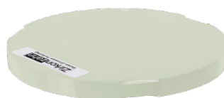
Figure 2 – Zirconia blank colored zirconia for the production of jewelry (e.g. rings, pendants) and other creative works. The final color is observable only after sintering. http://www.zirkonzahn.com/pt/produtos/materiais-fresaveis/zirconia-creative .
