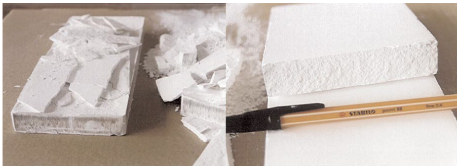
Figure 9 - Al 2 O 3 sample pressed without (left) and with (right) vacuum (Kaiser, 2007) [10]
