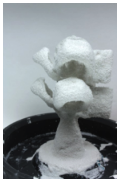
Sprinkled with alumina sand and dried
