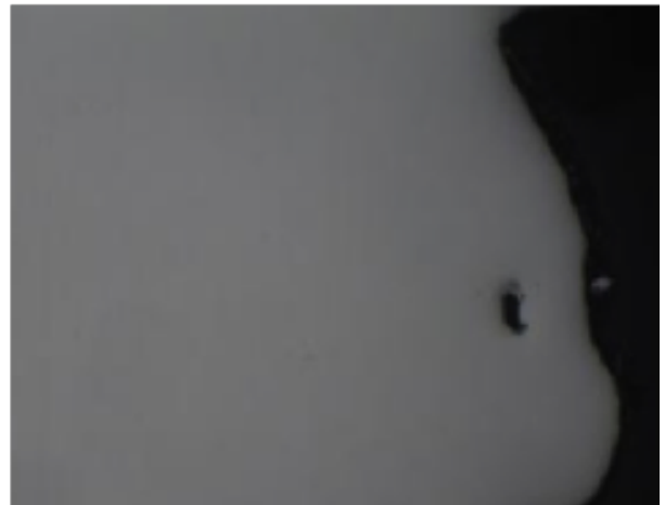
Figure 12b Sectioned Pt90Ir10 gas pore after HIP
