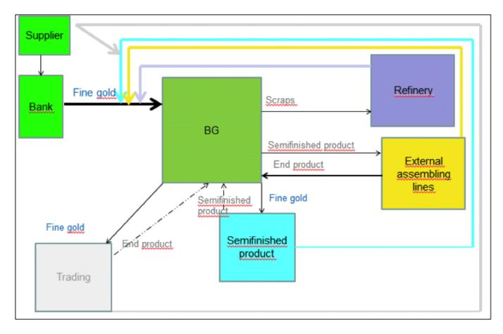
Figure 1 Metal flow diagram
