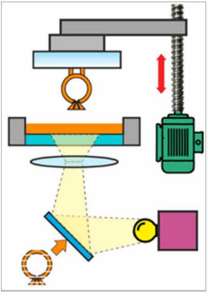
Figure 1 A schematic of the typical DLP process
