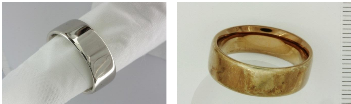
Figure 12: Bulk metallic glass ring as polish (left) and after wearing test of 52 days (right)
