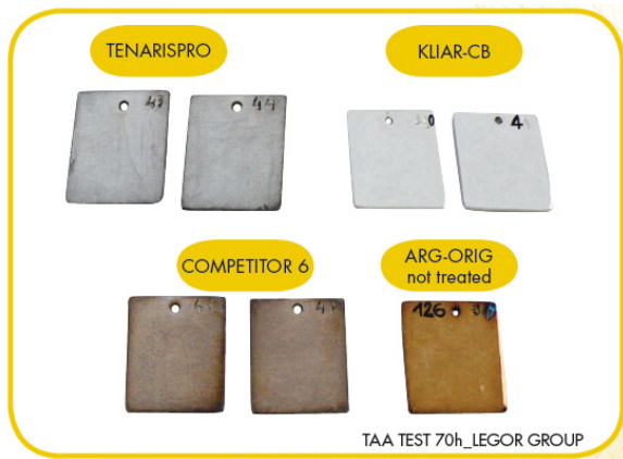
Picture 2. Oxidation resistance test (TAA test for 70h) for KLIAR-CB (the new transparent e-coating) and for most effective passivating agents on the market today in Sterling Silver sample-plates.
