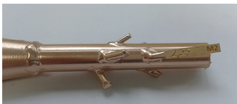
Figure 3 – 2nd identification plate for sprue recognition
