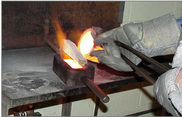
Figure 6: Producing a 1000g gold ingot
