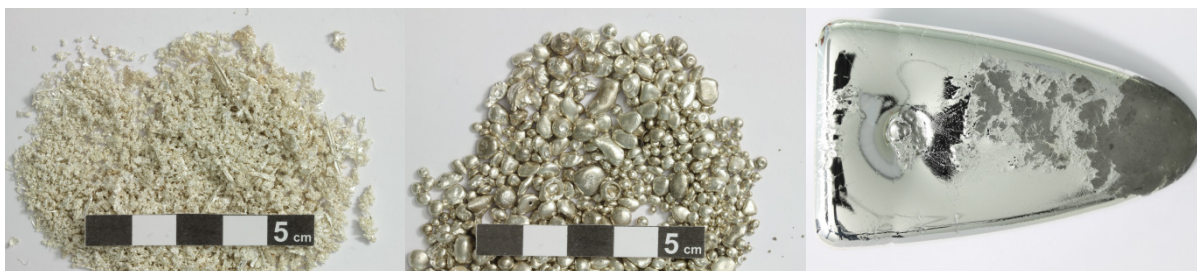
Figure 8 999 Ag raw material for melting. Left: Electrolytic silver, oxygen content 400 ppm. Center: Silver granules, oxygen content 250 ppm. Right: Vacuum-melted silver bar, oxygen content <10 ppm.
