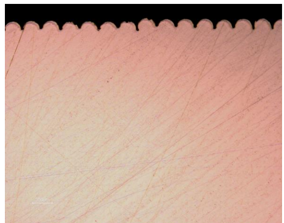
Figure 25 – Metallographic section of the piece with double laser scan
