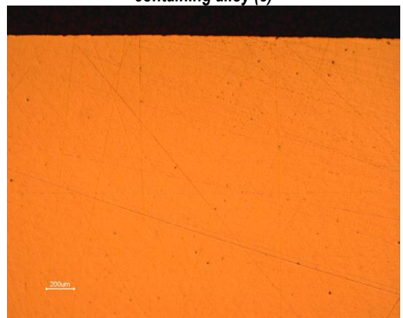
Figure 39 – Direct investment casting of the gallium containing alloy (3)
