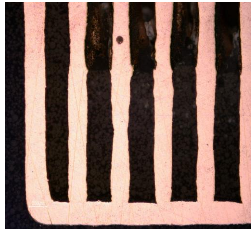
Fig. 14 – Vectors with 82.5 Watt power and 80 µs laser exposure time
