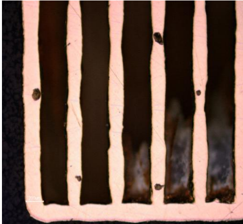
Fig. 11 – Vectors with 72.5 Watt power and 0.5 m/s scanning speed
