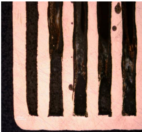
Fig. 13 – Vectors with 92.5 Watt power and 80 µs laser exposure time
