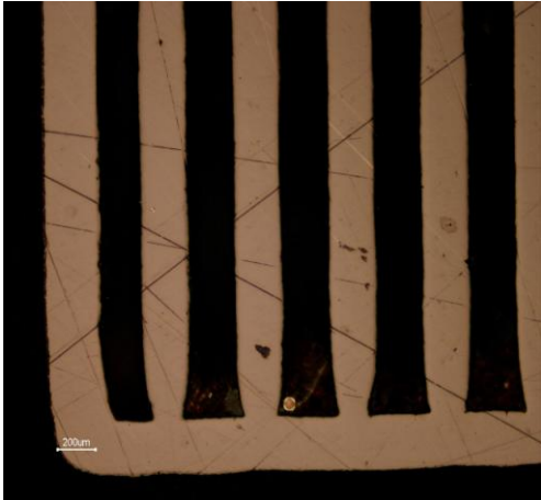
Fig. 5 – Vectors with 92.5 Watt power
