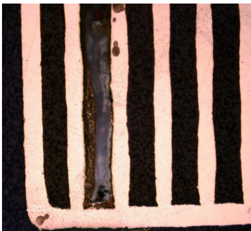
Fig. 15 – Vectors with 72.5 Watt power and 80 µs laser exposure time
