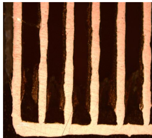
Fig. 16 – Vectors with 62.5 Watt power and 80 µs laser exposure time
