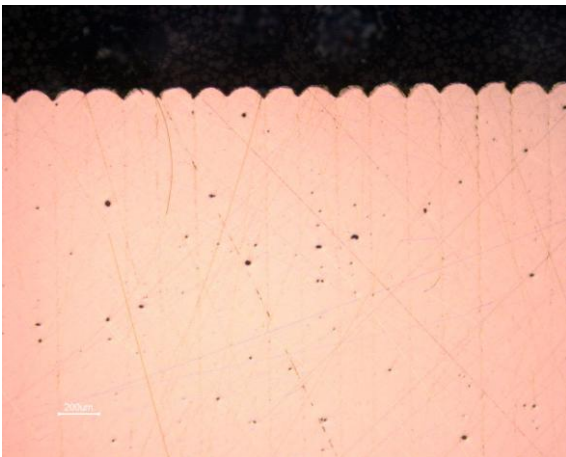
Figure 21 – Cross section of the vectors with 180 µm distance
