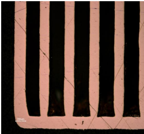
Fig. 7 – Vectors with 72.5 Watt power
