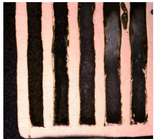
Fig. 10 – Vectors with 82.5 Watt power and 0.5 m/s scanning speed
