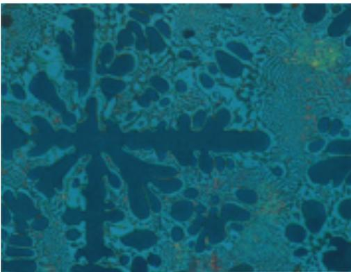
2. Microstructure of a 2 phase cast silver-copper alloy
