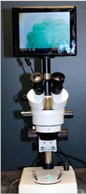
Figure 3 Our digital stereomicroscope
