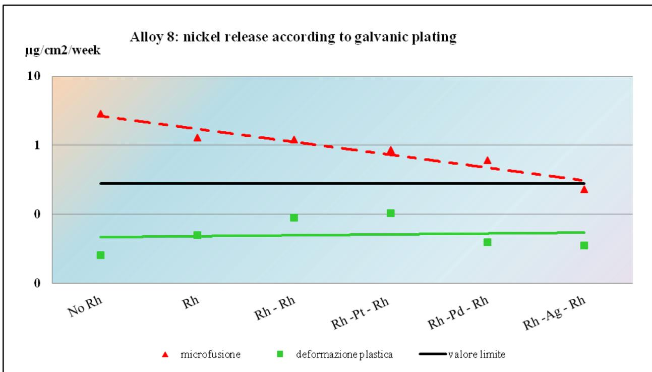
**Figure 5: nickel release for galvanic plating processes**
