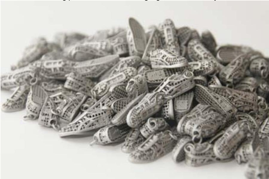
Figure 8 Example of geometrically complex fashion accessories produced using the FCubic technology
