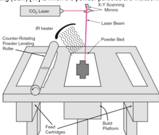
Figure 7 Diagram showing an example of powder bed laser technology
