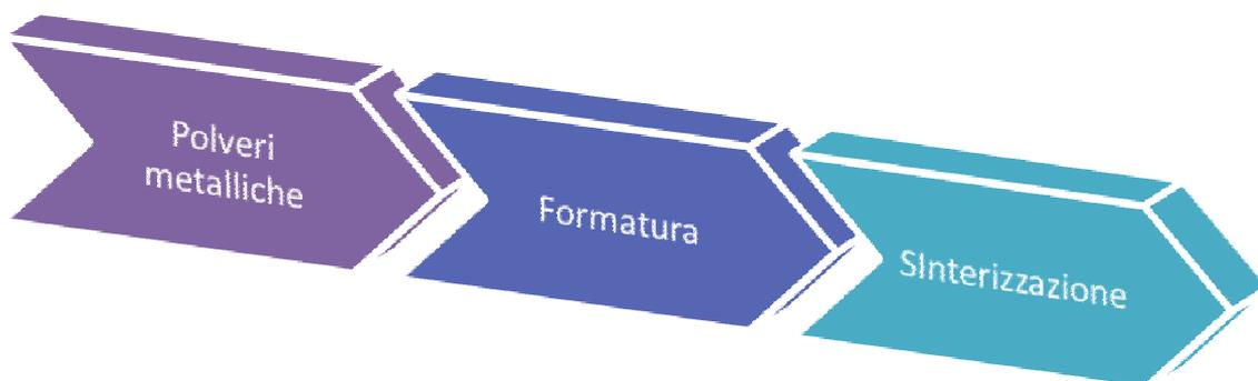
Figure 1 Process phases in Powder Metallurgy technologies
