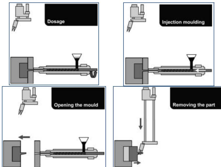
Figure 6 Diagram of the MIM injection process, the injection mixing stage, injection, mould opening and item extraction.
