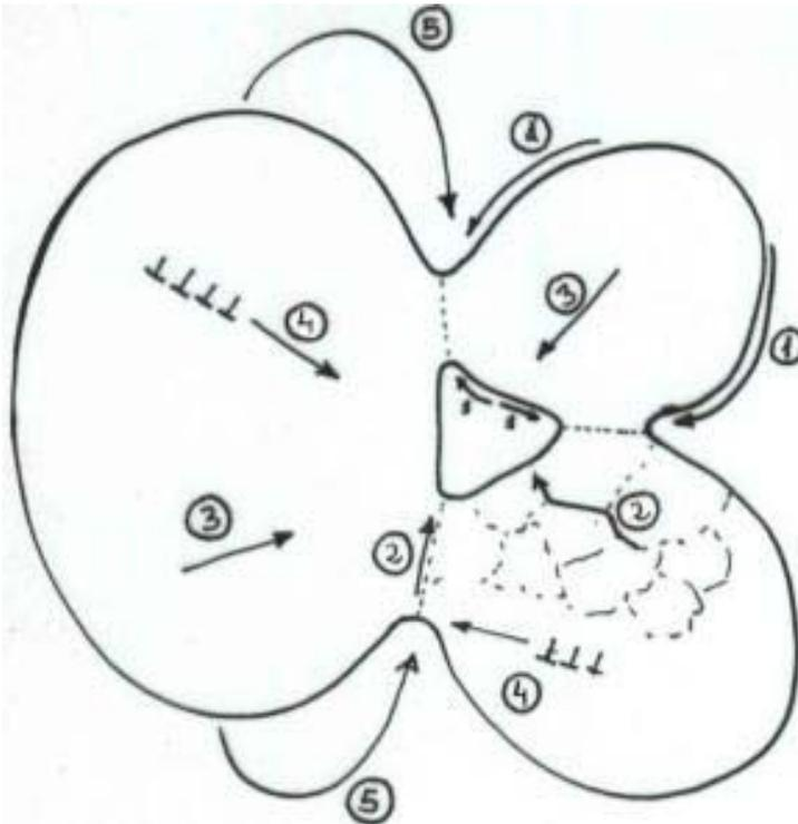
Figure 3 Diagram showing examples of scattering processes: superficial (1), grain boundary (2), volumic (3), plastic flow (4) and evaporation-condensation phenomena (5).
