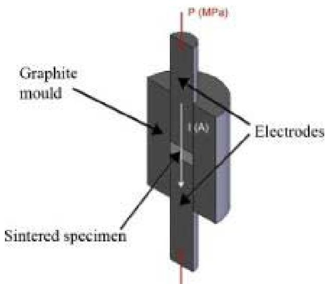
Figure 5 Diagram of a FAST device in which the electrodes also do the pressing.
