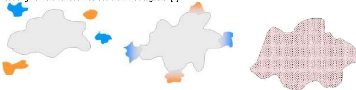
Figure 2 Diagram showing powders mixed mechanically, pre-alloyed by scattering and totally pre-alloyed.
