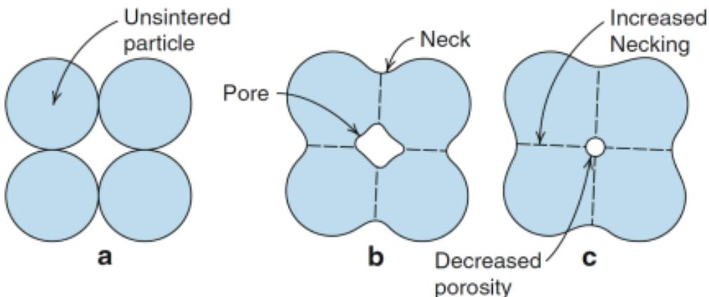
Figure 4 Sintering process of free particles (a), formation of sintering necks (b) and densification (c).
