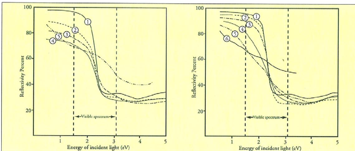
Assessment of the degree of whiteness of an alloy can be performed via the Yellow Index <sup>(6)</sup> (YI) which is a scalar number calculated from spectrophotometric data (in the same way as the CIELab coordinates). The Yellow Index derives from an index used for plastic (Standard D-1925).
