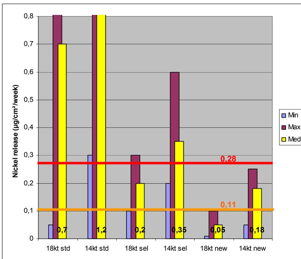
These interesting possibilities can provide greater guarantees of safety in terms of compliance with the limits established by the new EN1811:2011 standard, despite the inevitable fluctuations in release values depending on the specific situations of use.
